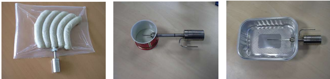
Fig. 1: The installation of sensors to determine the temperature in the product core
