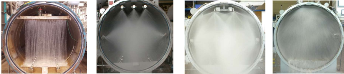
Fig. 2: Different spraying and cascading processes influence the temperature distribution in the autoclave. From left to right: simple cascade, water sprayer with simple nozzles, water sprayer with large twisted nozzles, and water sprayer with welded nozzles.
