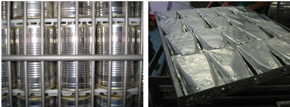
Fig. 1: Accessories for optimizing the temperature distribution are e.g. whaffled spacer mats (left) or special trays for product placement (right).
