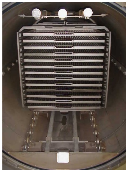
Fig. 3 „Rack“-Cage with inserted trays
