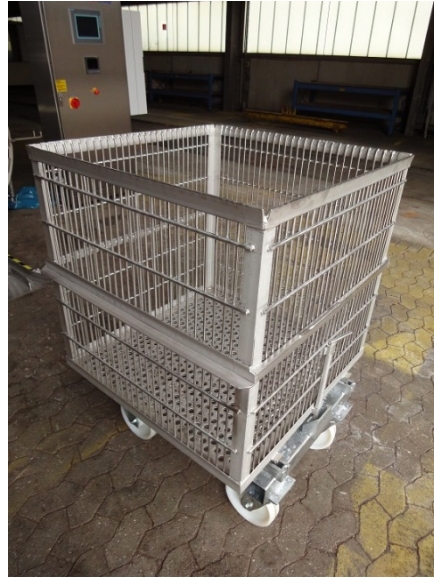
Fig. 1 Cages made from perforated galvanized steel sheets (left) and from stainless steel grid (right)
