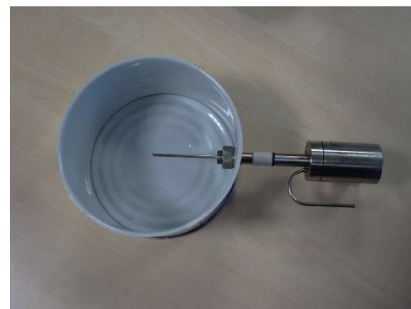
Fig. 4: Preparation of a container for the heat penetration measurement
