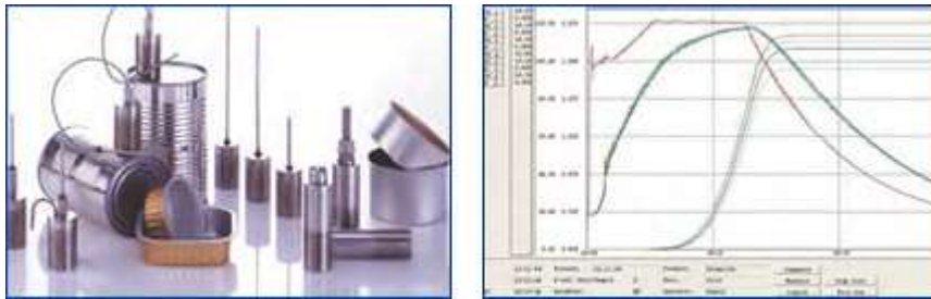
Fig. 1: Different sensors, adapted to the product and its packing (left) are used in the validation. The measurement results are documented in a non-manipulable way and displayed in graphics (right).
