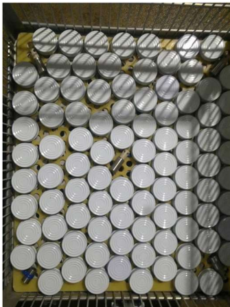
Fig. 3: Fixation of the loggers between the water filled containers
