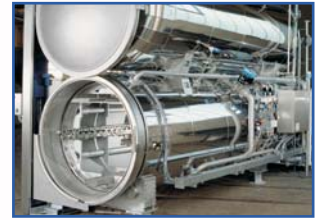
Vollwasser-Autoklaven Full Water Immersion Retorts
